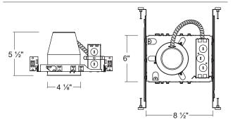
L-tech 4" LED GU10 dedicated IC housing, H400LGICQA is designed for new construction using GU10 LED Max 10W and for direct contact with insulation.
